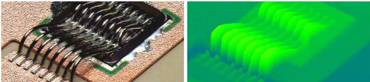
*The results of Viscom innovation: 3D wire bond inspection of thick wire on DCB substrate, as a real image and a height image*
