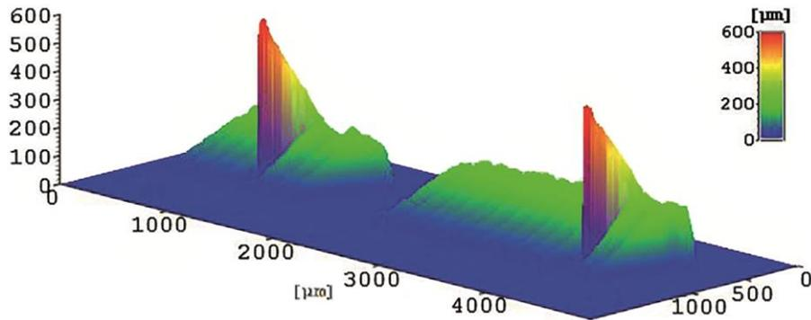
*3D information aids not only the inspection of heights and distances. Through the precise determination of the course of the wire, it also enables the inspection of specified wire lengths.*
