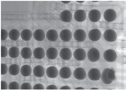
Head-in-pillow defect on BGA component
