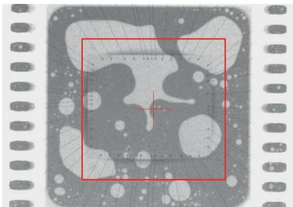
Surface soldering with voids
