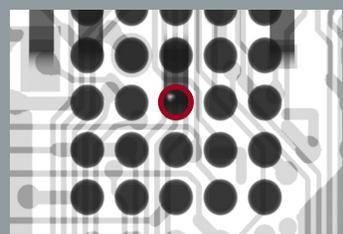
2D image of a BGA: structures from the back side are present in the image
