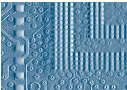
Slice image of a printed circuit board section with BGA
