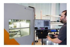
The Viscom X-ray inspection system inspects the number and size of voids at the SMT Technology Center
