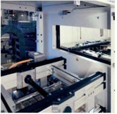
With the new Heavy Flex handling options, even extremely heavy inspection objects can now for the first time be inspected fully automatically in the process line using 3D AOI and 3D AXI. (Photo: Viscom AG)
