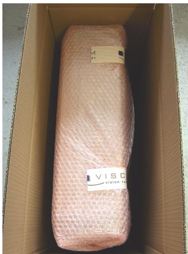
7. Protect the two upper edges of the computer with a suitable cushioning material.
